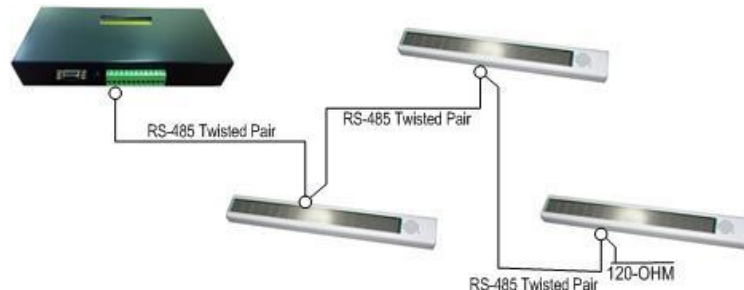
Multi-Drop RS-485 cabling and 120-ohm termination
